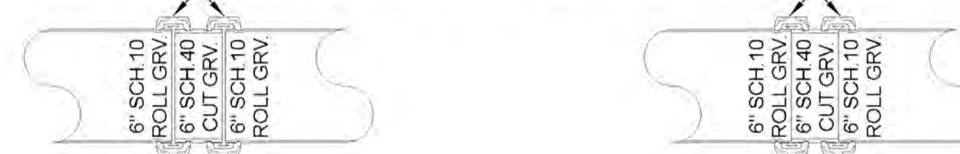
UN-EXPANDED PIPE (2) COUPLINGS AT MAX PARALLEL DEFLECTION EXPANDED PIPE (2) COUPLINGS AT ZERO PARALLEL DEFLECTION
